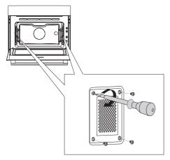
1 Undo the four screws on the cover. Remove the cover and the glass.
